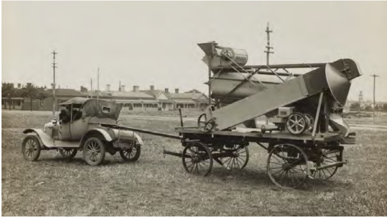
Seed cleaner, grader, and bagger ready for delivery during the 1920s. This rig may have been photographed on the open, reclaimed land opposite the factory.
