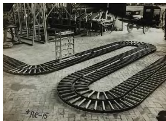
A Roller conveyor layout being prototyped in the Schumacher factory in 1925. Source: Museums Victoria Collections.
